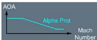
In the case of Alpha Prot undue activation due to blocked AOA probes, the flight control laws order a continuous nose down pitch rate that may not be stopped with backward sidestick inputs, even in the full backward position. If the Mach number increases during a nose down order, the AOA value of the Alpha Prot will continue to decrease. As a result, the flight controls laws will continue to order a nose down pitch rate, even if the speed is above VLS.
