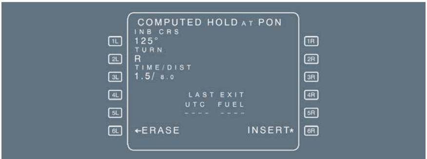
If the holding pattern is not in the database, the FMGC designs a holding pattern and proposes it to the pilot. The associated data consists of default values that the pilot can modify.
