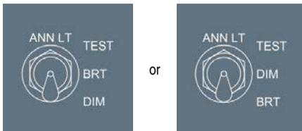
**TEST :** All flight deck annunciator lights turn On.
