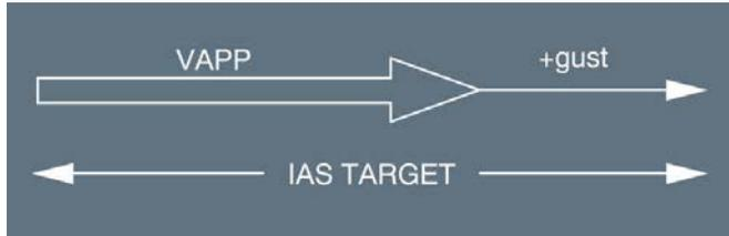
The gust is the instantaneous difference between the CURRENT HEADWIND COMPONENT and the TWR HEADWIND COMPONENT. It is always positive (or equal to zero for no wind or tailwind).
