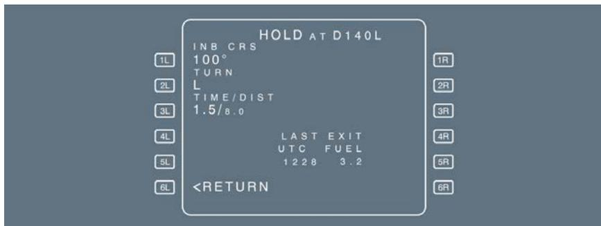
If the pilot inserts into the active flight plan a holding pattern that is manually-corrected from a hold defined by the FMGS, the screen displays a “HOLD AT...” page. The 2R field displays REVERT TO DATABASE or REVERT TO COMPUTED to restore the database data, if necessary.
