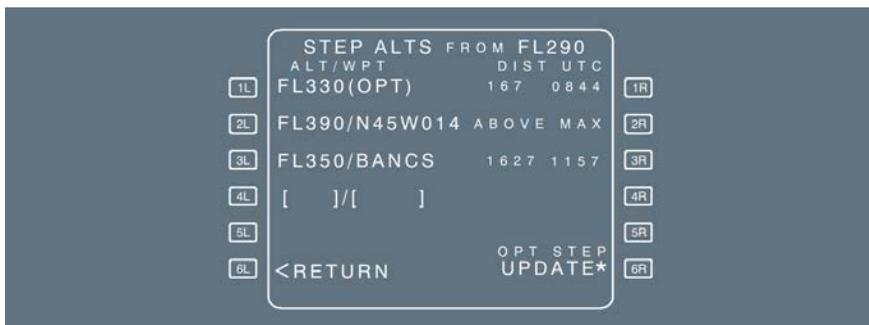
The computed (OPT) step replaces the initially inserted step position, and is then considered at a fixed geographic position. Savings are no longer displayed, and the UPDATE\* prompt replaces the INSERT\* prompt. This prompt allows the crew to update the (OPT) step position, considering possible F-PLN or inserted wind changes.
