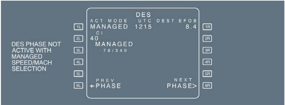
If the flight crew reverts to the **SELECTED** speed/MACH mode during descent, the profile is not modified and the aircraft flies the same profile at the FCU selected speed/MACH value.
