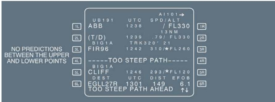
When the aircraft reaches the beginning of the too steep path segment, the FM recomputes the VDEV using an idle segment from the end of the too steep path segment.
