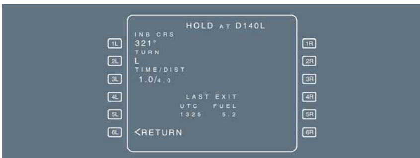
The FMGS predicts the estimated time and amount of fuel remaining at which the aircraft must exit holding, so as to comply with the fuel policy specified on the fuel prediction page. When the aircraft enters the holding pattern, the FMGS revises all predictions and assumes the aircraft will fly one turn of the holding pattern. All predictions are revised for one more holding circuit at holding fix overfly.
