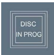
Note: After the release of Mobile Com pushbutton, the DISC IN PROG light comes in blue and remains on until the total disconnection of the system.
