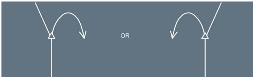
For shorter range scales, and if the procedure turn or the holding pattern is in the next or the active leg, the display shows the full circuit or pattern.
