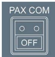
**OFF** : The Cabin Connectivity system is cut-off. When the pushbutton-switch is released, the OFF light comes on in white.
