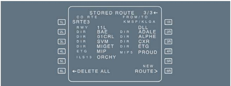
This page displays up to 5 routes, stored by the pilot. The stored routes are listed and numbered in the order of insertion. The number is displayed in the upper right-hand corner of the page.
