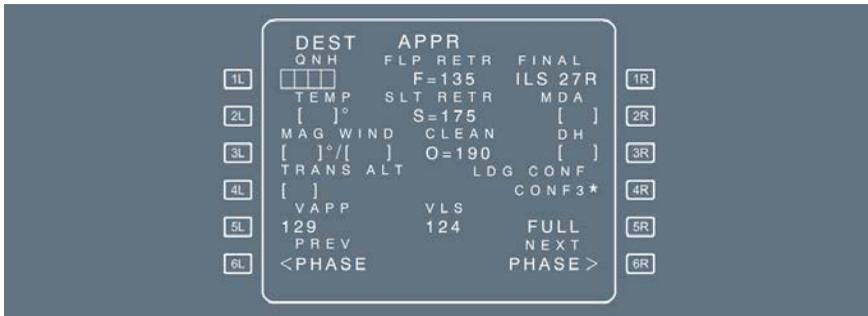
The scratchpad displays “ENTER DEST DATA” if the approach page is not completed when the aircraft is 180 NM from destination.
