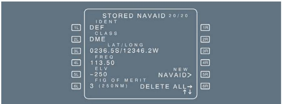
A number in the upper righthand corner of the screen shows the relative order in which the NAVAIDs were stored. (For example, 3/7 means the third out of the seven stored).
