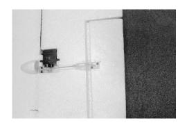
2. Push the wing rod into the wing as shown. Fix the main wing panel to the fuselage. Use a tool to fix and install the main wing onto the fuselage.
